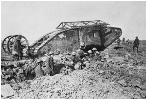
Mark I tankBritish Mark I tank with anti-bomb roof and “tail,” 1916.
